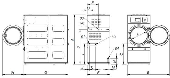
01 Refrigeration water inlet (supply network) 1/2" 02 Refrigeration water outlet (hot) 1/2" 03. Power supply 04 Drain 3/4" 05 Ethernet connection
