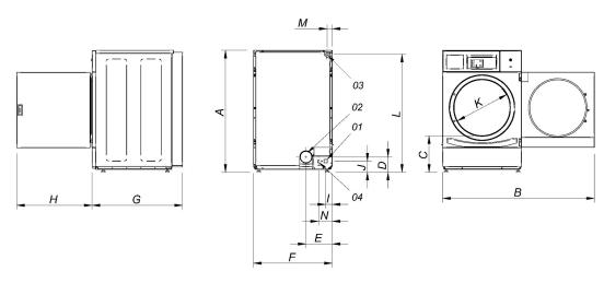
01 Power supply 02 Fumes output Ø 100 03 Gas inlet 1/2" 04 Ethernet connection (only TOUCH control)
